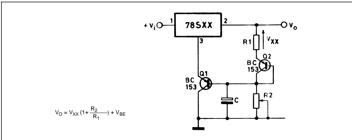
NOTE:  $Q_2$  is connected as a diode in order to compensate the variation of the  $Q_1$   $V_{BE}$  with the temperature.  $C$  allows a slow rise time of the  $V_O$ .
