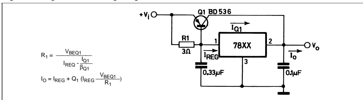
Figure 16: High Output Current with Short Circuit Protection
