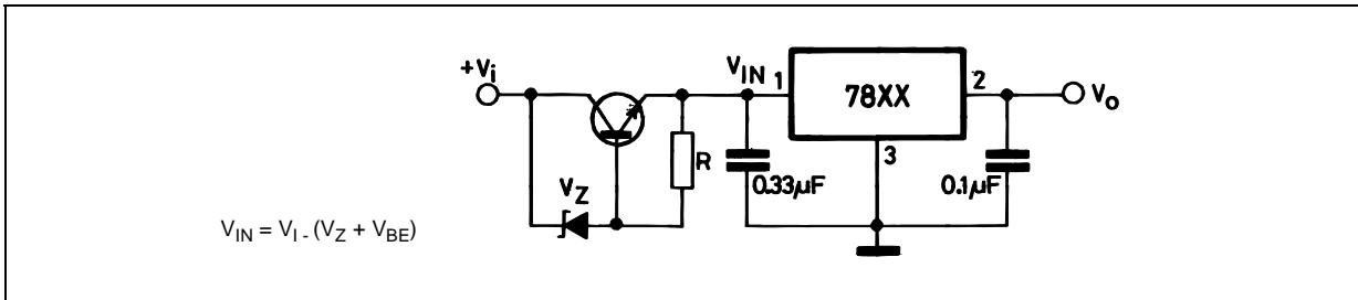
**Figure 22: High Input Voltage Circuit**
