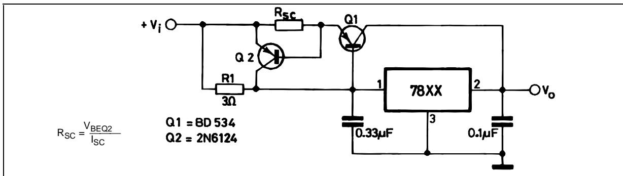
Figure 17: Tracking Voltage Regulator
