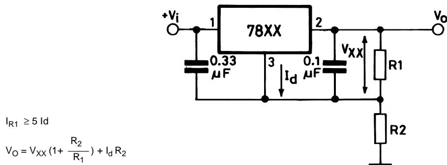
**Figure 13: Adjustable Output Regulator (7 to 30V)**
