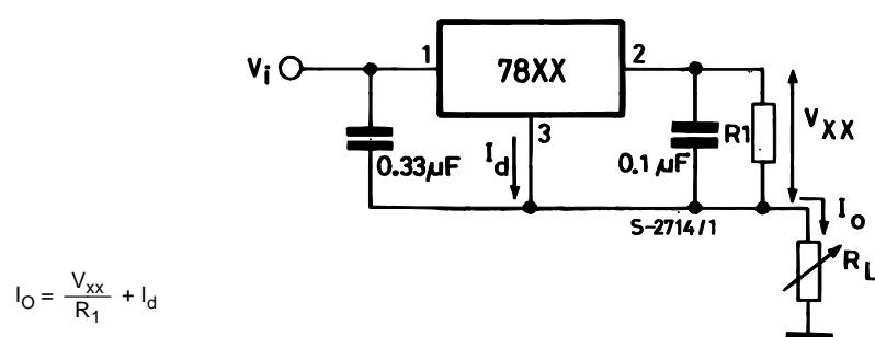
**Figure 12: Circuit for Increasing Output Voltage**
